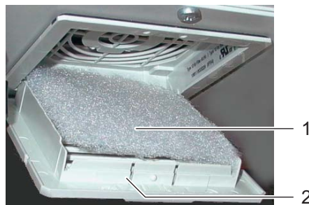
figure 5-16 Exchanging the lower filter mat
