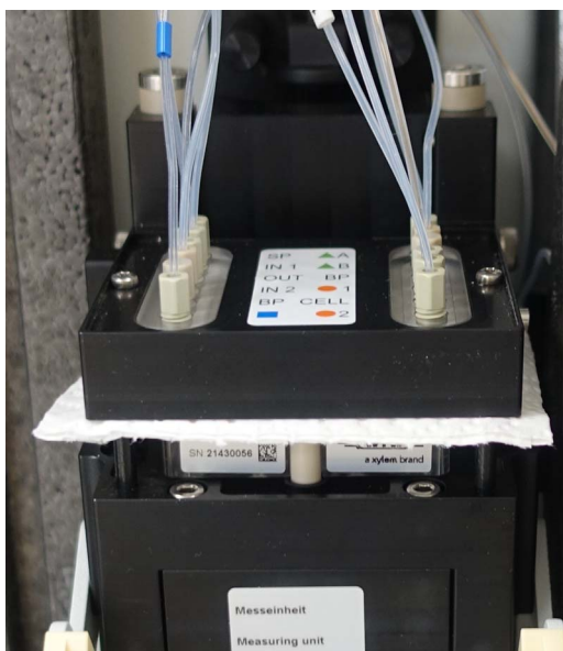
figure 5-2 Removing the liquids remains with absorbent, lint free paper
