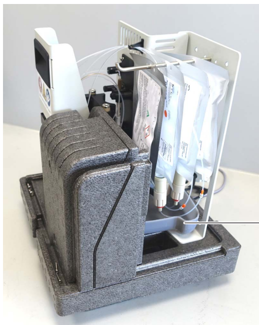
figure 5-7 Position of the collection tray in the measuring unit (under the ChemBags)
